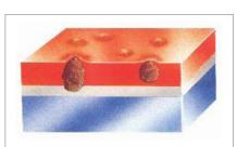
Fisheyes are small rounded indentations that resemble fisheyes. This is caused by foreign substances that do not blend with paint.
